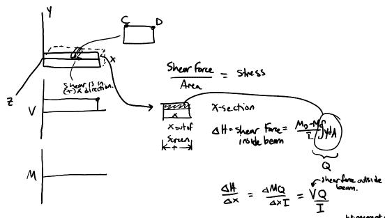
Shear Flow 5 hear force a ching over whole length Shear Stress - Shear force per unit area
