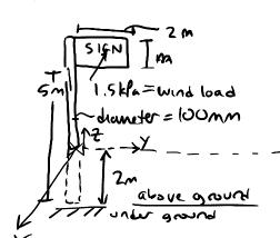
wind is blowing down x axis in neg x direction.
