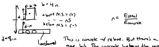
gap ble The concrete between the newhal surface court hold fersion.
