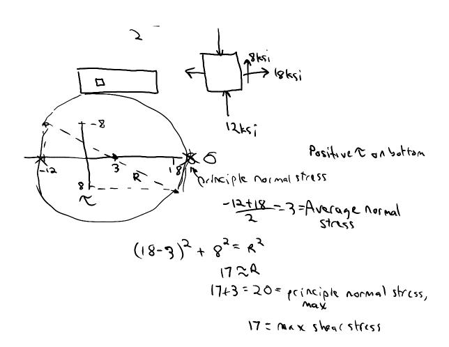
There's one orientation where the normal stress is by itselfno shear stress
