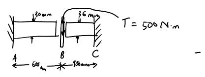
Maximum shear stress in 2 shafts
